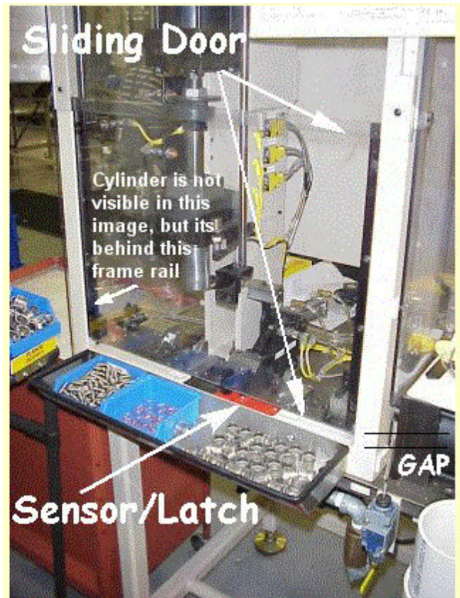
Great Idea #037 (Gravity drop door w/whisker switch for cycle initiate)
