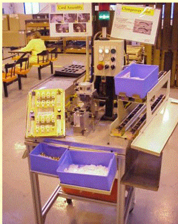
Great Idea #034 (Load fixture and manually pull head over fixture)
